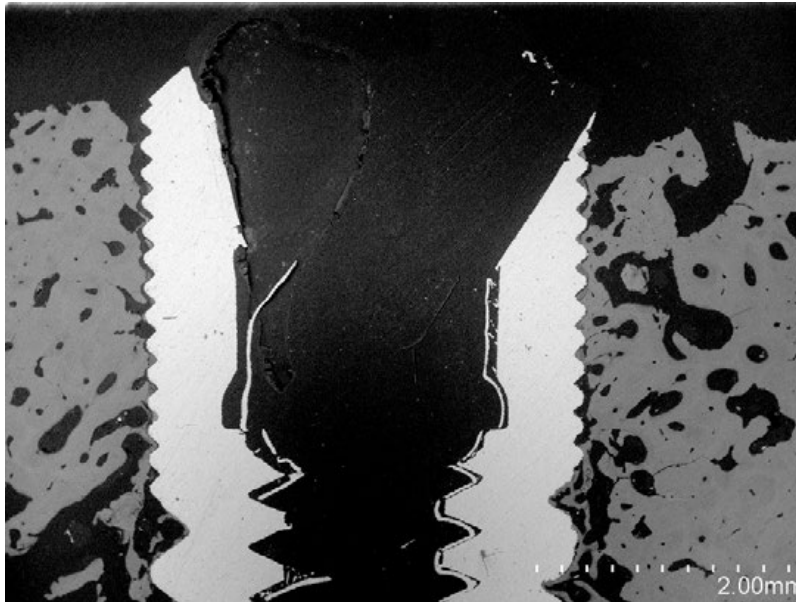
Figure 4-16 Dental implant at 8 weeks in an animal model. This transcortical section was imaged with secondary electron diffraction (backscatter mode) to show continuous adaptation of bone along the small threaded portion on the cortical region.
